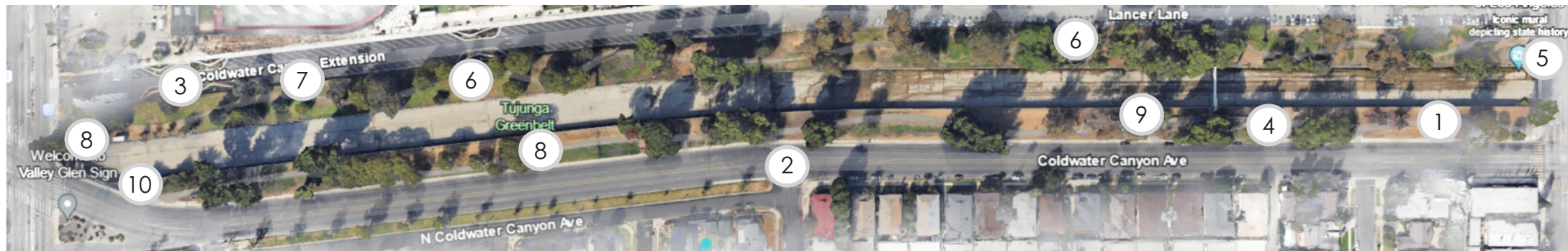
2 Calming traffic by narrowing Coldwater Canyon, adding crosswalks, and creating a bermed buffer for cyclists.
