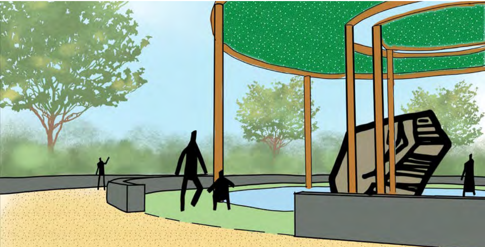
Corten Steel circular shade structure fitted with sun shade. Sun shade material permeable to allow for water drainage in case of rain.
