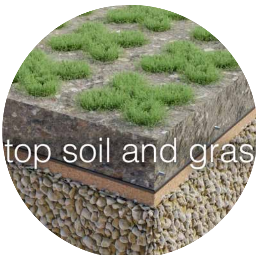
Grass crete section revealing materials & permeability.
