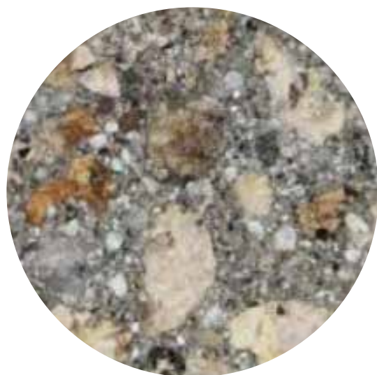
Lithocrete aggregate can be created in different colors and textures to be used on the main plaza.
