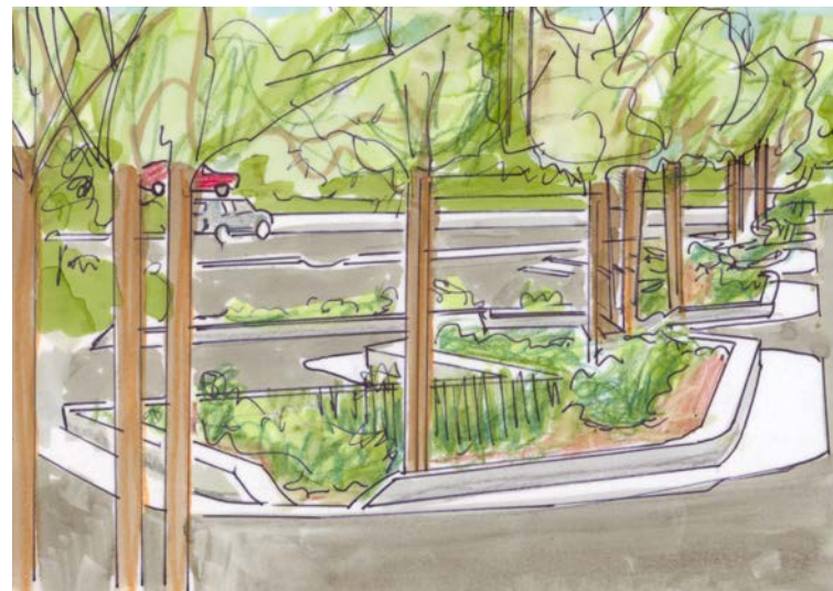
Curbing with planters and trees that absorb heat and water.
