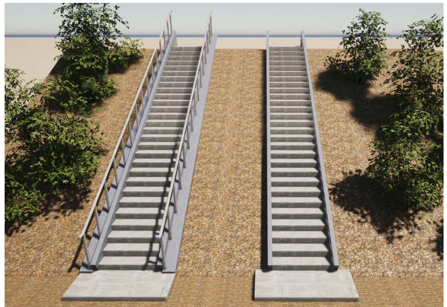
Stair model. Right side, original. Left side, improvement with a handrail in concrete to the side of the original granite that could be implemented to the existing stairs that preservationists do not want to remove or tamper with in any way.
