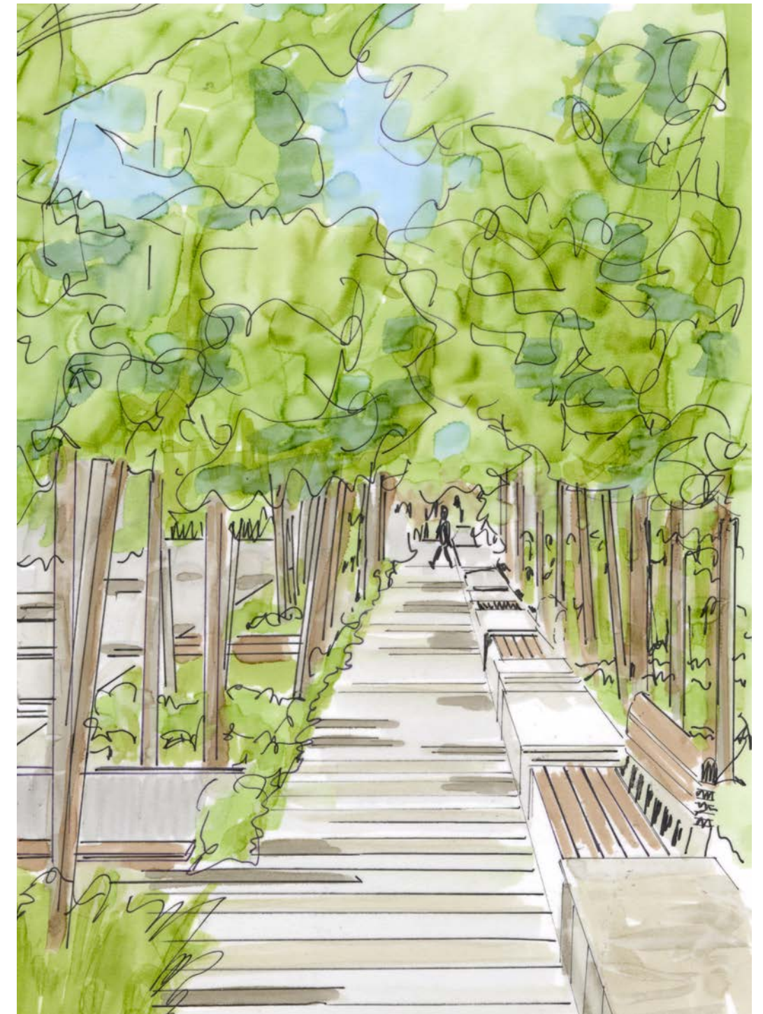
Center swale with permeable paving for water retention, and shaded bench seating.
